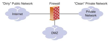
Figure 13-1 Typical Firewall Configuration Before FWLB
